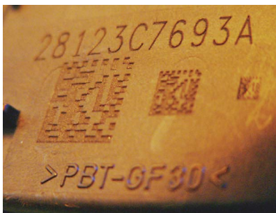
A laser can etch a permanent Data Matrix symbol and alphanumeric characters into a component. Symbols can conform to several size standards.
